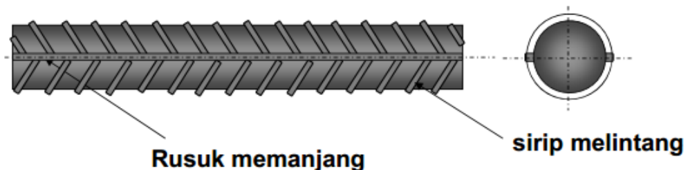
Gambar 3.2 - Baja tulangan beton sirip/ulir (BjTS)
