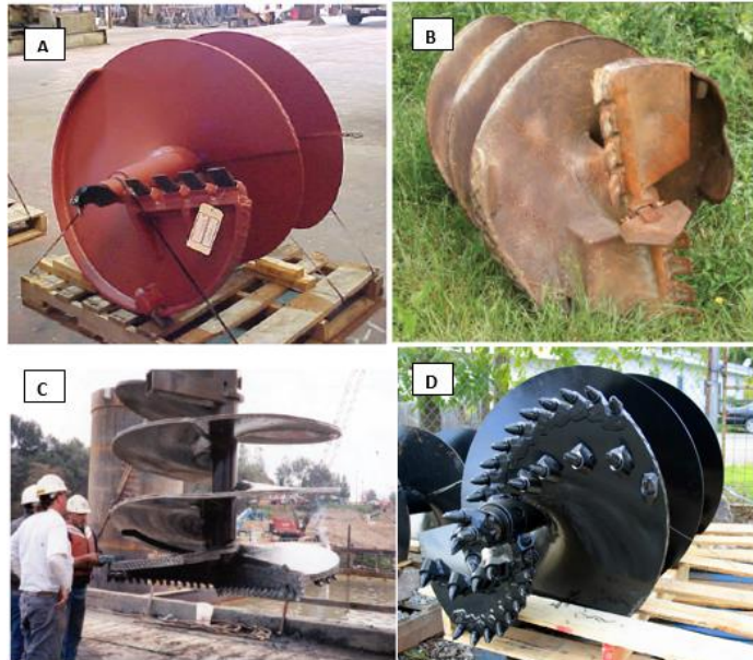
Gambar 4.26 - Beberapa jenis auger; A) Single flight auger ; B) Double flight auger ; C) Large diameter auger dengan double cutting edge ; D) rock auger
