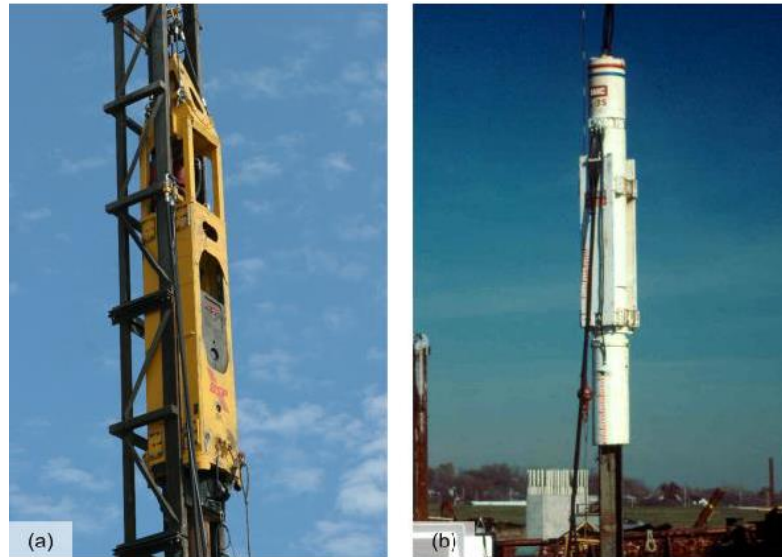
Gambar 4.16 - Ilustrasi peralatan hydraulic hammer ; a) single acting hydraulic ; b) double acting hydraulic
