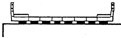
Flat Plate Bridge with precast slabs
